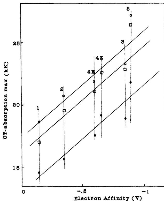
**Figure 1.** CT absorption maximum ( $10^3 \text{ cm}^{-1}$ ) of the EDA complexes of tetrasubstituted olefins with donors vs. their reduction potentials: (●) complexes with *N,N*-dimethylaniline, (□) complexes with *N*-ethylcarbazole, (○) complexes with hexamethylbenzene.
