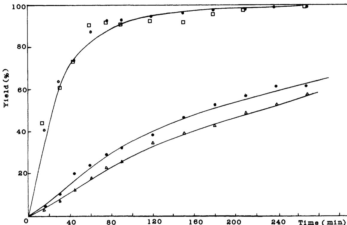
Figure 3. Time-conversion curves of the polymerization of *N*-vinylcarbazole initiated by **1** or **1-Cb** at 30.5 °C in dichloromethane.  $[1] = 0.01$  M,  $[NVCZ] = 0.22$  M, (O) polymer, (●) yield of cyclohexane **7**.  $[1-Cb] = 0.01$  M,  $[NVCZ] = 0.21$  M, (□) polymer, (Δ) yield of cyclohexane **7**.
