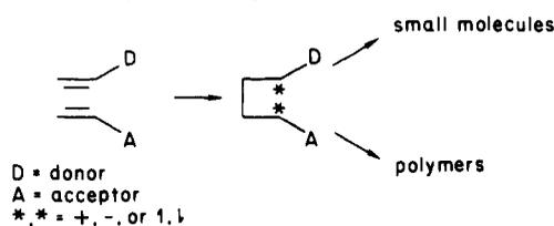
Zwitterionic tetramethylenes are postulated to initiate ionic homopolymerizations, while copolymers arise from initiation by biradical tetramethylenes.
