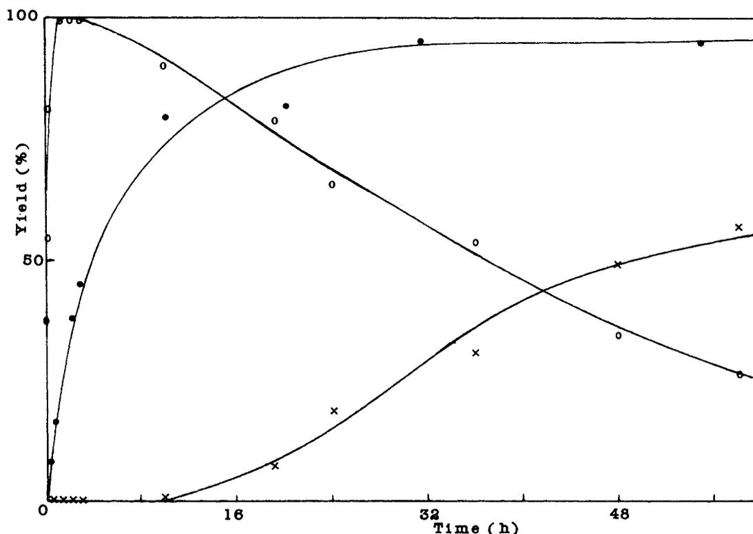
Figure 4. Time-conversion curves for the TCNE-NVCZ-3 reaction in dichloromethane at 30.5 °C [ $3$ ] = 0.10 M, [NVCZ] = 0.40 M, (●) polymer yield calculated for 0.3 M NVCZ, (○) yield of cyclobutane 3-Cb, (×) yield of *trans*-1-butene derivative 3-Bu calculated for 0.10 M 3.
