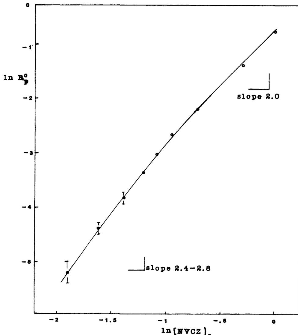
Figure 6. Initial polymerization rates of NVCZ initiated by cyclobutane 3-Cb with varying [NVCZ] in dichloromethane at 30.5 °C, [3-Cb]<sub>0</sub> = 0.05 M.
